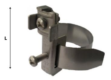
GS A2 grounding strip provides an earthing junction between  $\emptyset$  17 - 48 round pole or cable and 1 x 16 mm<sup>2</sup> - 2 x 25 m<sup>2</sup> grounding cable.
